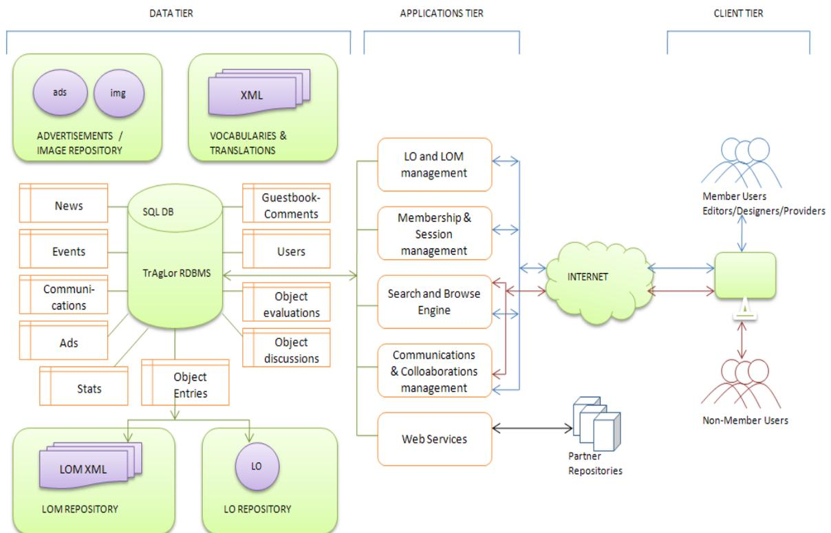
Figure 1. System architecture of TrAgLor
